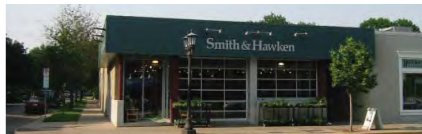
Buildings should show a minimum of 30% window coverage on each front that faces a street
