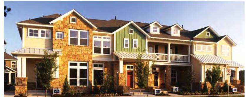
The exterior of attached/townhome dwelling units shall include a variation in building materials which are to be distributed throughout the building facades
