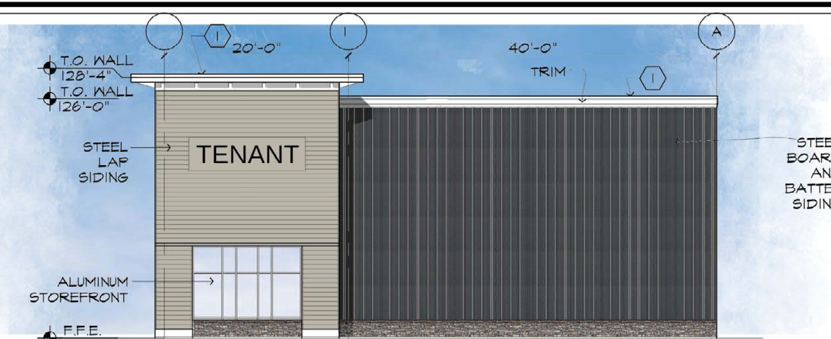
2 NORTH ELEVATION - OFFICE/WAREHOUSE
